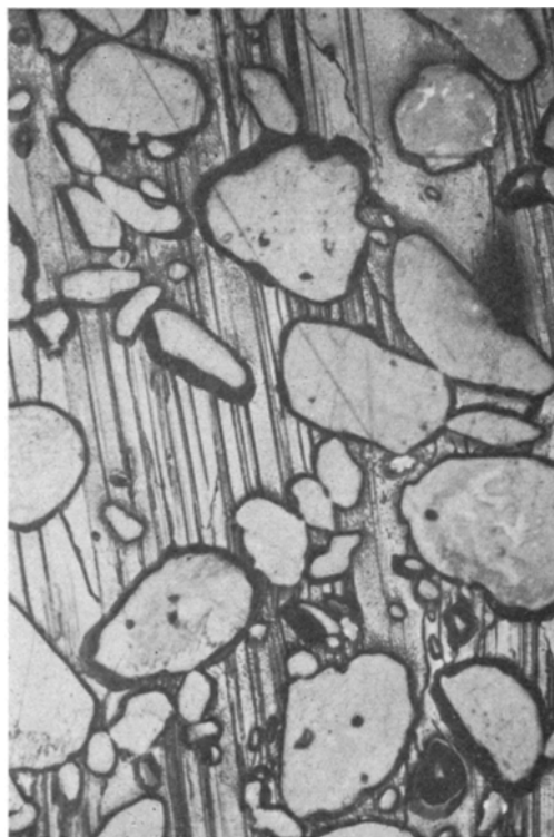
Figure 1 Polished Composition B. Bromoform etch ( \times 200 ).
